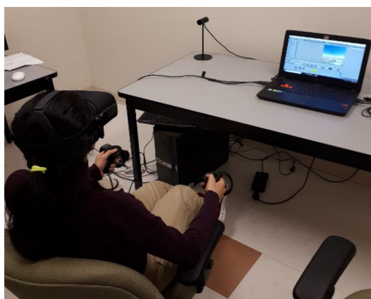
Fig. 15 Hardware setup, depicting a participant taking part in the experiment. The chair position was fixed to avoid real body rotation
