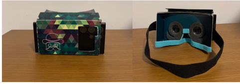
Fig. 2. Google Cardboard Device with front cut-out to expose middle camera, blue foam on face and nose bridge, and head strap.
