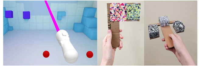
Fig. 1. (Left) Virtual controller with selection ray; four floating shapes represent controller and selection apparatus tracked markers. (Right) Cardboard Controller in right hand and selection apparatus in left.
