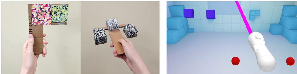
**Figure 1: Left: Low-Fi VR Controller in right hand and cardboard piece with selection markers in left hand depicting the Marker selection method. Right: VR view of the controller with sphere and cube objects indicating tracking statuses of markers**
