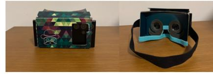
**Figure 5: Google Cardboard Device with front cutout and foam modifications.**
