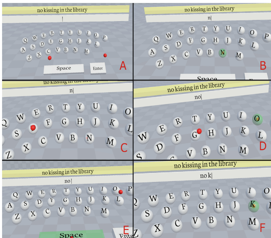
Fig. 3. Fluid intersection keyboard (FLIK). (A) Shows the phrase to be transcribed before the user has entered any text. (B) The user selects the character ‘n’ by moving his right hand through it so that the red selection cursor touches and goes through the character as seen in (C) where the sphere cursor is now behind (and partially occluded by) the ‘n’ character key sphere. (D) Again, shows the same right hand having looped around the bottom of the keyboard and selecting the ‘o’ character key sphere from beneath. (E) As the right hand exits the character ‘o’, the left hand now moves through the spacebar to select a space character. (F) User continues in this manner selecting the next character.
