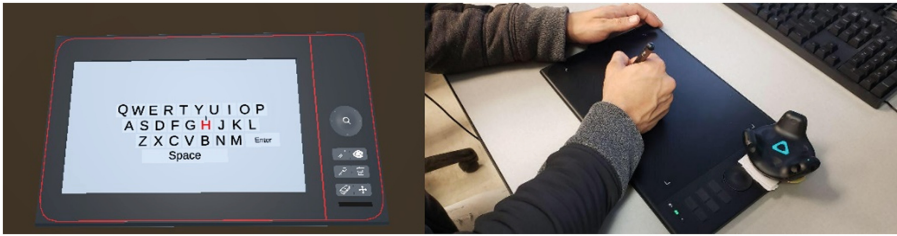
Fig. 1. (Left) The VR view, showing the QWERTY soft keyboard. The “H” key is highlighted to reflect that the stylus is currently hovering over it. (Right) Participant performing the experiment with the Tablet and Stylus.
