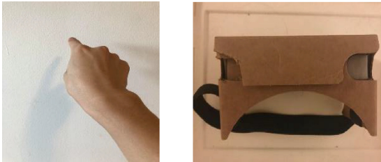
Fig. 12. Left: Tap gesture. Right: Modified Google Cardboard with both left and right-sided button
