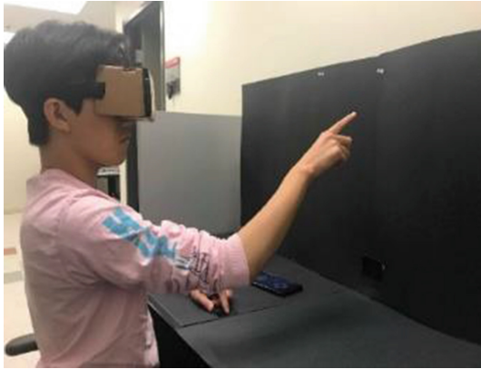
Fig. 1. Participant performing a selection task wearing a Google Cardboard HMD. The button can be seen at the top-right of the device. No other external controller is provided.
