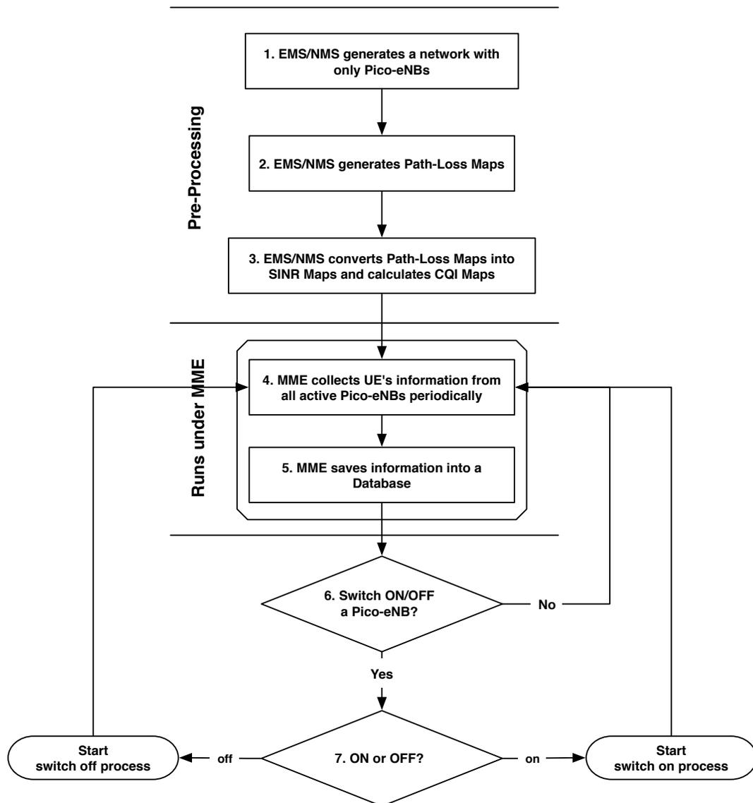
**Figure 4.12:** The enhanced centralized switch on/off algorithm
