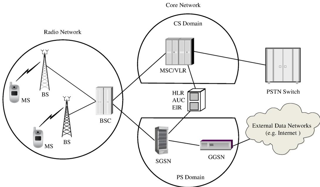
Figure 2.1: Architecture of 2.5G cellular networks
