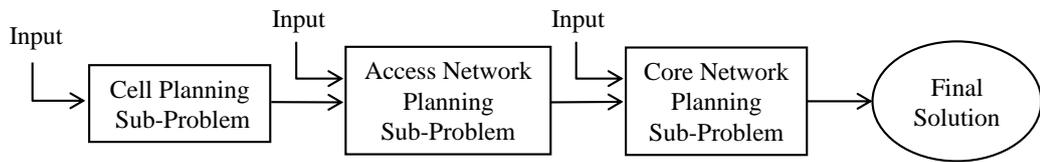
Figure 2.3: Sequential approach for UMTS planning sub-problems [4]
