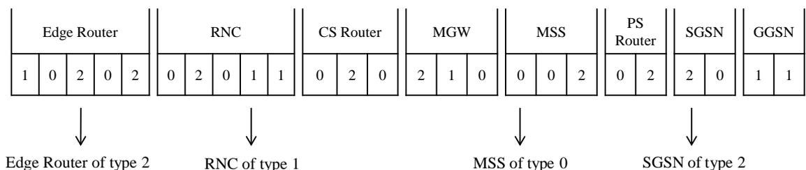
Figure 3.4: Example of the NE-Type vector
