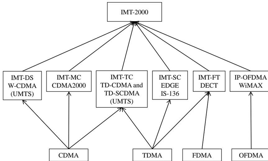
Figure 2.2: IMT-2000 radio interface standards [3]
