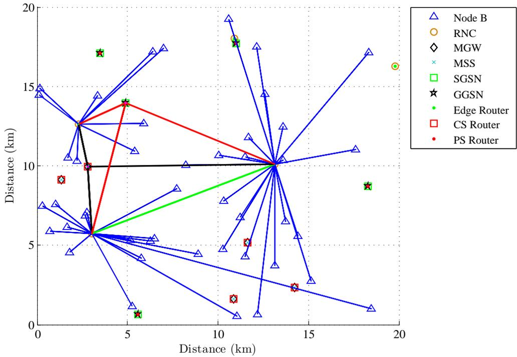
Figure 4.3: Solution for the illustrated problem obtained with TS
