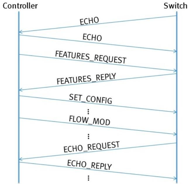
Figure 2.2 OpenFlow and Switch protocol exchange process
