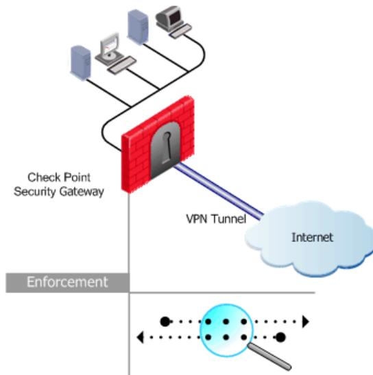
Figure 3.3.a Traditional Fire Wall with Statement Inspection solution
