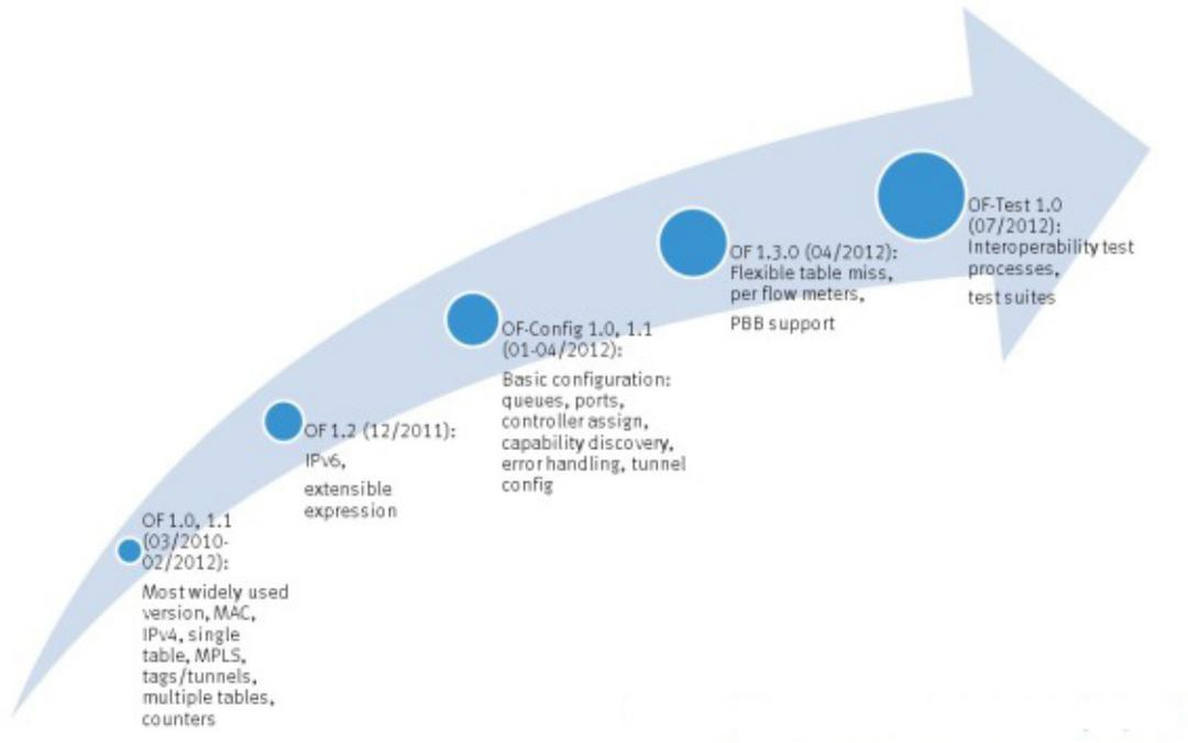
Figure 2.1.a OpenFlow specification development process
