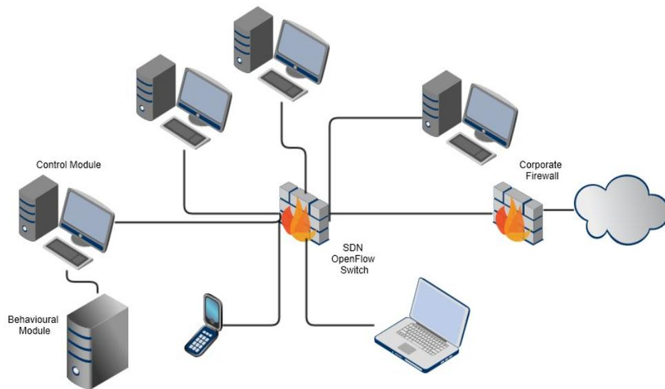
Figure 3.3.b OpenFlow Switch controls traffic of broadcast domain
