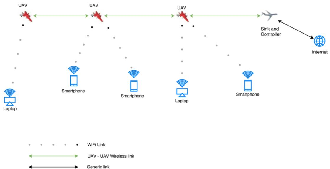
Figure 1.1: UAV-UAV and UAV-User communications
