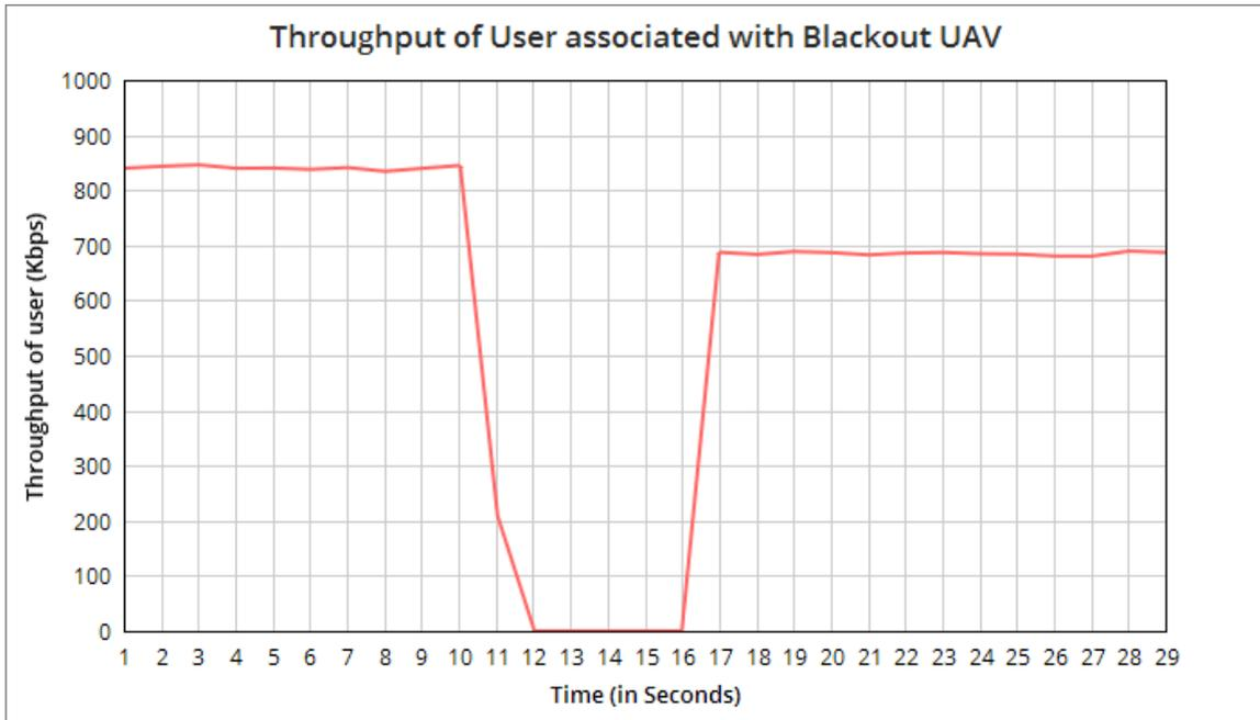
Figure 4.24: Throughput of user associated with blackout UAV
