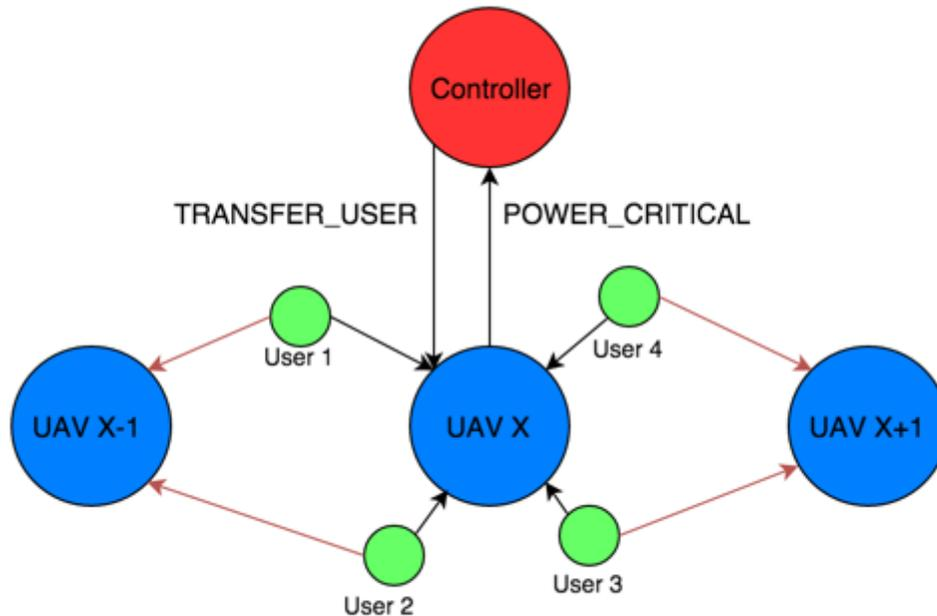
Figure 3.16: Handovers due to critical power level
