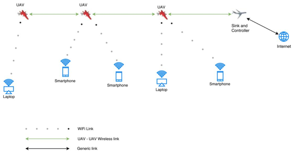
Figure 3.1: Overall network architecture
