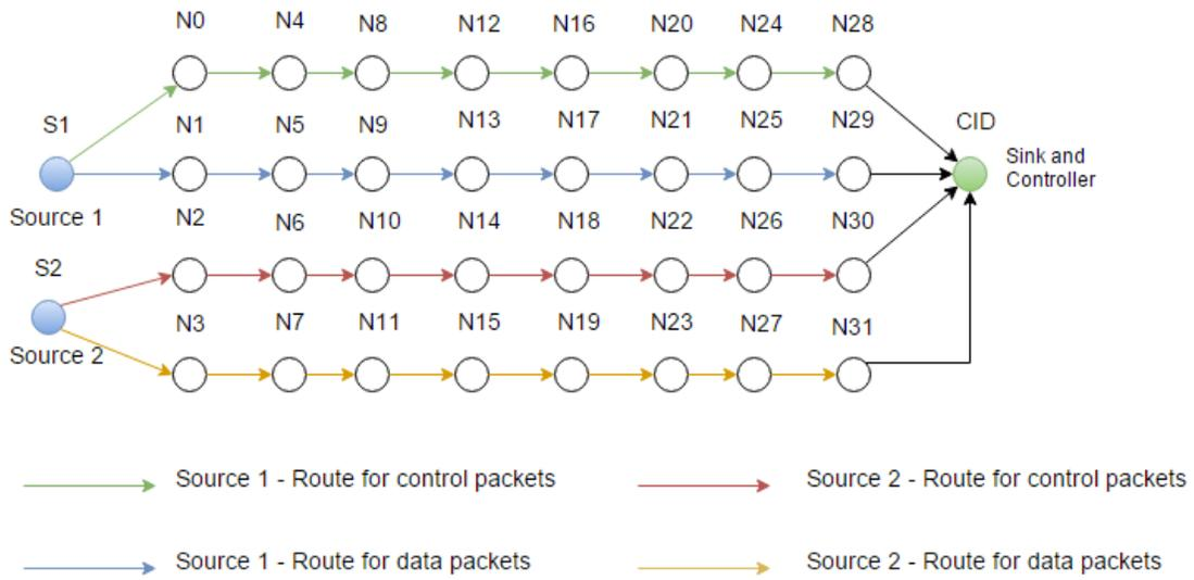
Figure 4.5: Experiment with 4 tier network consisting of 2 sources and 1 sink
