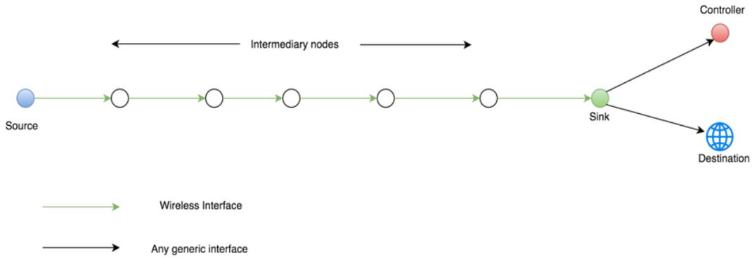
Figure 4.1: Linear topology for simulation
