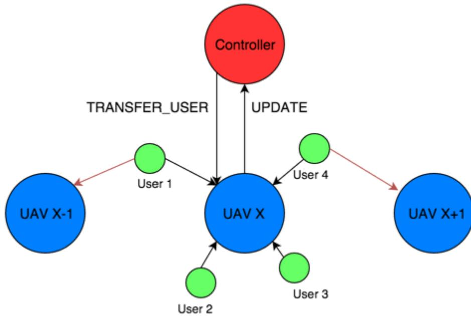
Figure 3.17: User transfer due to traffic spike
