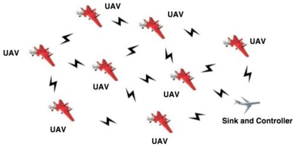
Figure 3.2: UAV-UAV communication backbone
