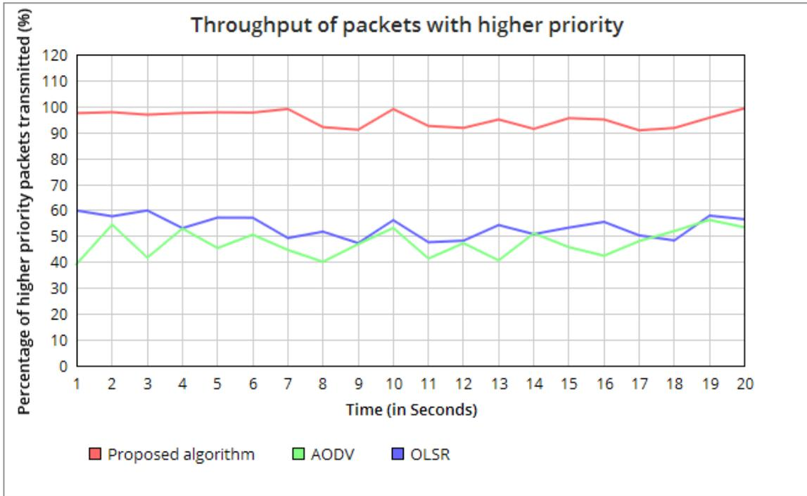
Figure 4.7: Priority packets successfully transmitted
