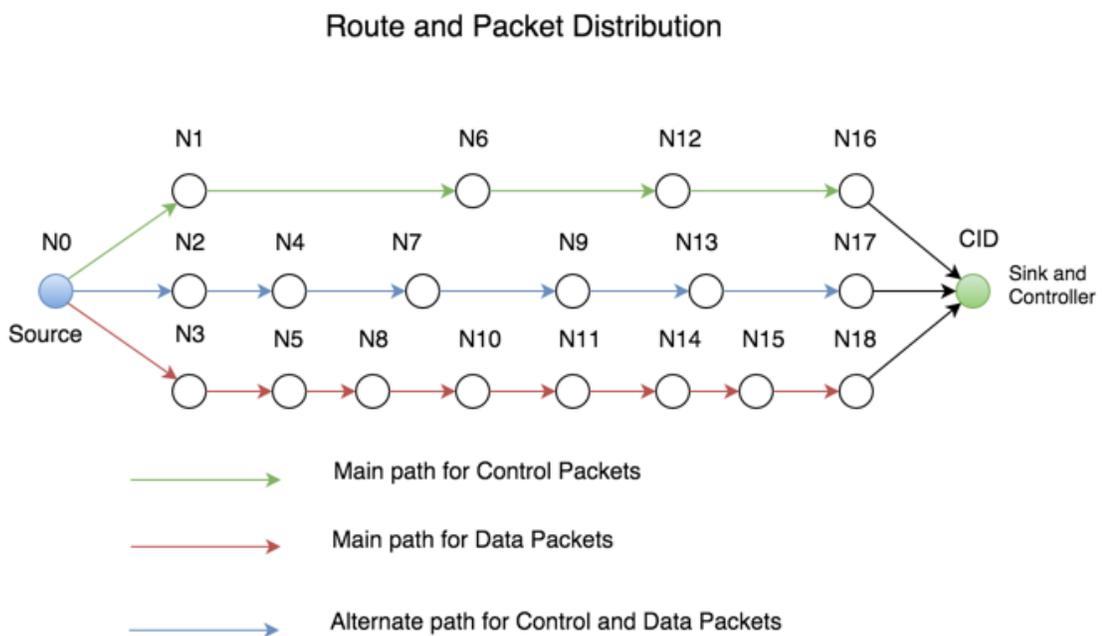
Figure 3.8: Paths for different priority levels assigned by the controller
