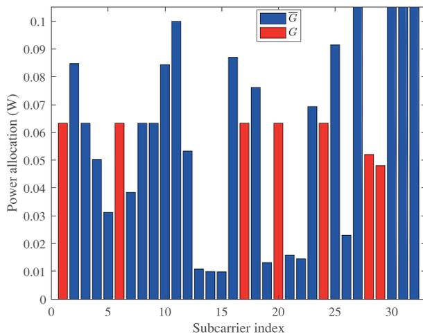
Fig. 8. Subcarrier and power allocation in the second phase.
