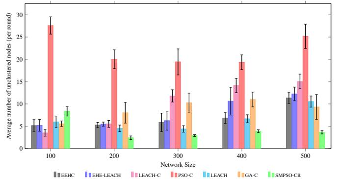
Figure 4: Average number of unclustered nodes per round for  $WSNs\#2$
