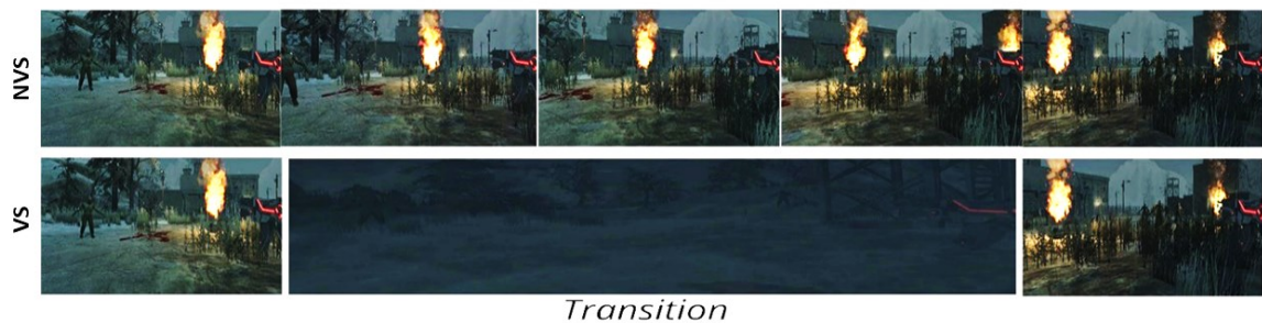
Figure 8 The top row of images shows a standard (non-snapping) viewpoint rotation. The second row shows the same rotation with our viewpoint snapping technique enabled. A fast transition eliminates the intermediate frames: meaning the rotation becomes discrete,
