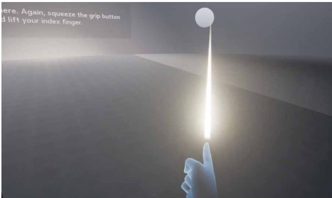
Figure 11: The Oculus Rift tutorial showing a virtual representation of the user's hands using ray casting to point at an object (Oculus, 2018).
