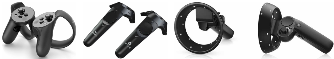
Figure 10: Various VR controllers. From left to right – Oculus touch, HTC Vive, Dell Visor controller (“Dell Visor,” 2018; “HTC Vive Controller,” 2018; Oculus, 2018).
