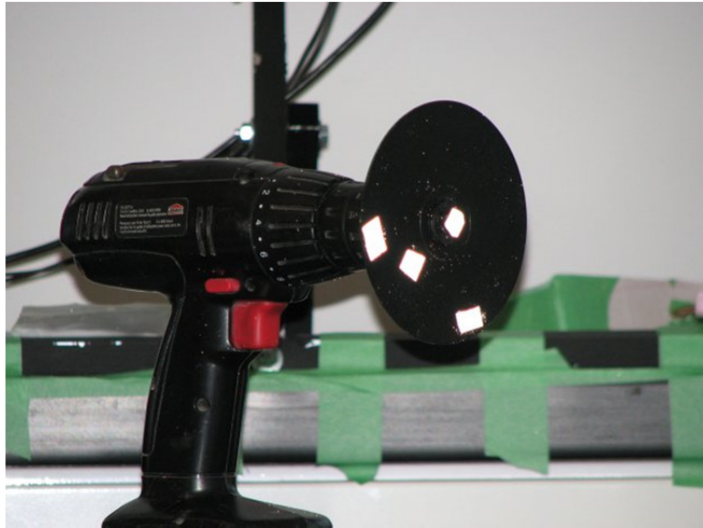
Figure 3-3. Rigid body mounted on a drill.
