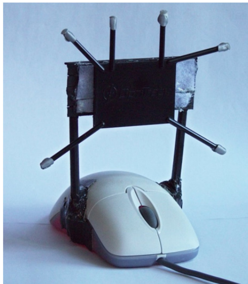
Figure 3-5. Mouse with optical tracking markers mounted.
