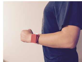
Figure 4. The wearable device used in this study (TI Sensortag).
