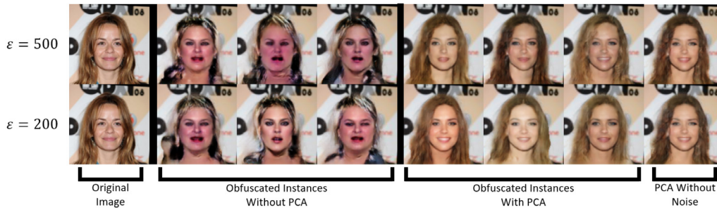
Fig. 7. A comparison of obfuscation with and without the use of PCA to control the application of the noise. The instances which do not use PCA demonstrate darkened facial features and distortions in skin tone, hair style and facial expression. The final column is included as a point of reference to show the visual impact of the dimensionality reduction from PCA without the application of noise.
