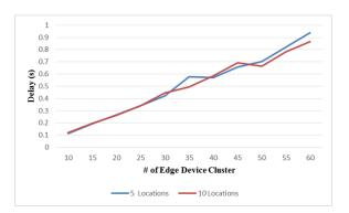
Figure 4.17: Delay comparison for different number of possible locations using the trade-off method
