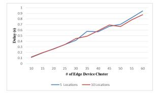
Figure 4.15: Delay comparison for different number of possible locations using the weighted sum method
