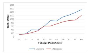
Figure 4.20: Traffic comparison for different number of possible locations using the trade-off method
