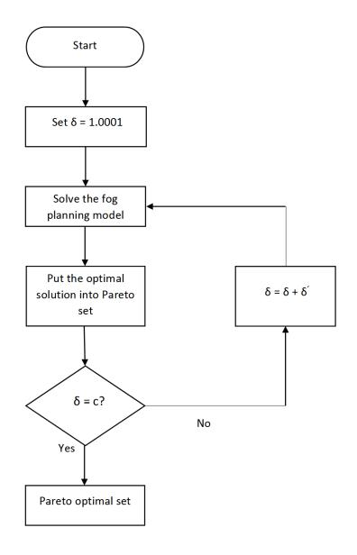
Figure 4.3: Steps to solve the FPP with the hierarchical method
