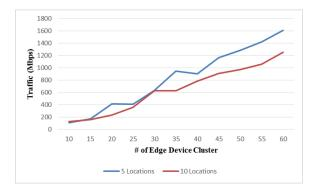
Figure 4.19: Traffic comparison for different number of possible locations using the hierarchical method
