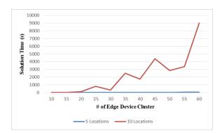
Figure 4.22: Solution time comparison for different number of possible locations using the hierarchical method
