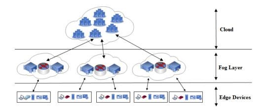
Figure 2.1: Reference architecture for fog computing
