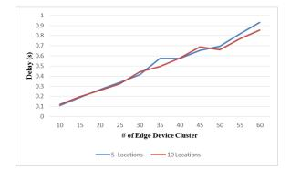
Figure 4.16: Delay comparison for different number of possible locations using the hierarchical method
